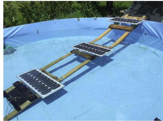
Fig. 17. Thermal management of PV panel by water submersion, [35]
