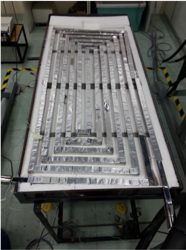
Fig. 36. Special spiral absorber design of PVT panel, [56]
