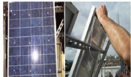
Fig. 9. PV-PCM cooling system for free-standing PV panel, [24]
